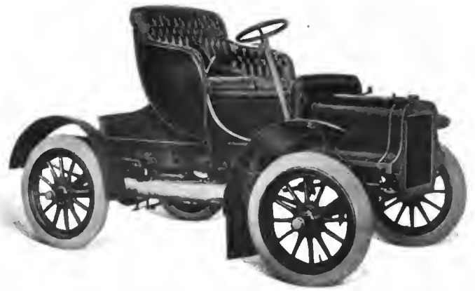
CADILLAC 10-HORSEPOWER CHASSIS, WITH RUNABOUT BODY AND TURTLE BACK.
